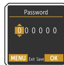
Use the buttons (12) ▲ or ▼ to select the **number**. Use the button ► to enter the next input field. Confirm your entry with the **OK button (10)**.
