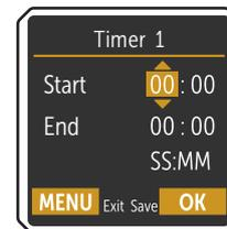
Use the buttons (12) ▲ or ▼ to select the **hours**. Use the button ► to enter the next input field. Select the **minutes**. Confirm your entry with the **OK button (10)**.
