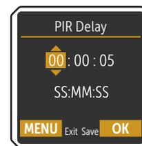
Use the buttons (12) ▲ or ▼ to select the **hours**. Use the button ► to enter the next input field. Select the **minutes and seconds** accordingly. Confirm your entry with the **OK button** (10).
