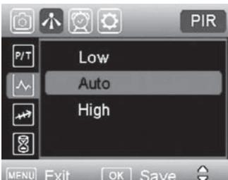
**PIR Sensitivity:** The camera will react on movements and temperature changes. Select this mode, press „MENU" to get the menu of trigger mode.
